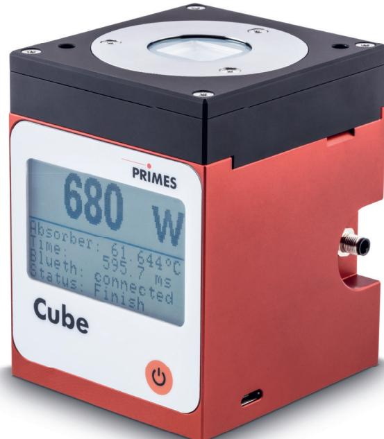
Its palm-sized design allows it to fit easily into the very tight spaces inside machines for use in laser material processing and it is designed to handle very high power densities. For some high-power applications, the irradiation is too intense for standard power meters and will destroy the coating on the absorber. The Cube M, however, can measure power densities of up to 250 kW/cm<sup>2</sup> with power of up to 2 kW!
